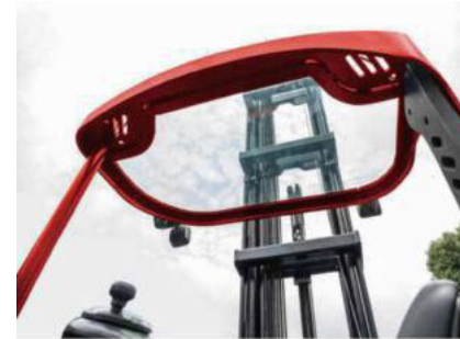
Optional: Overhead guard with panoramic glass offers excellent visibility for elevated location.
